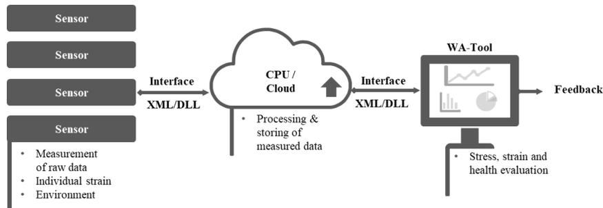
**Fig. 3.** System structure and concept of the component interaction of the WA project.
